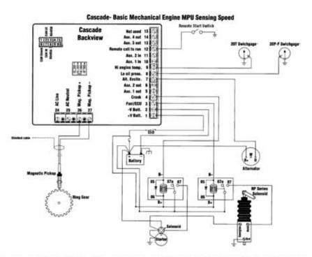
NOTE: This diagram represents typical wiring scenario, and is not the schematic to the panel.
